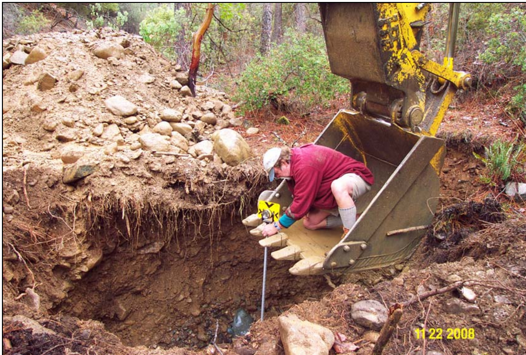
Photo 15. Surveying depth to bedrock and the water table surface in an excavation pit.
